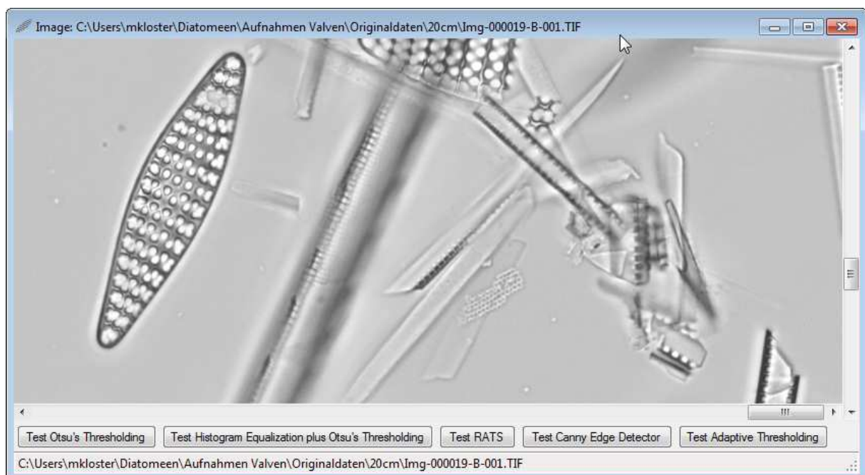
Fig. 6 Image window showing a brightfield micrograph of a valve and buttons for testing segmentation procedures
