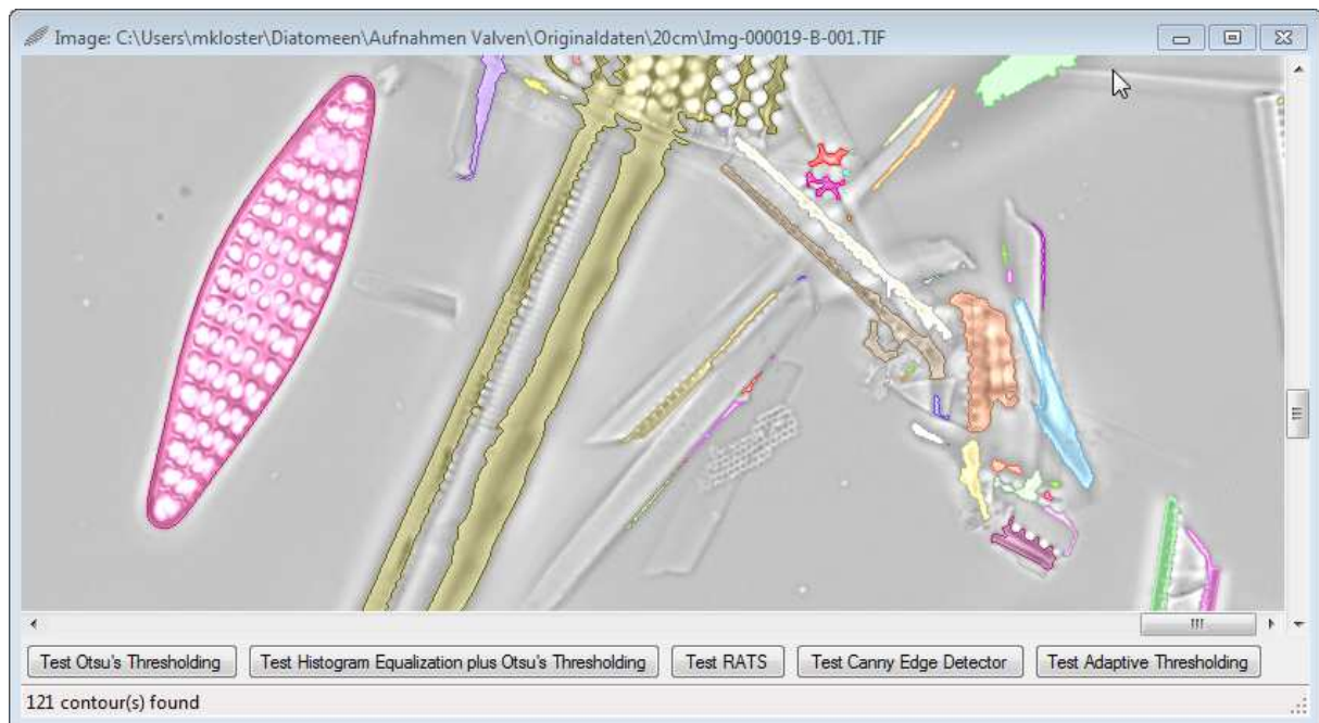
Fig. 9 Typical result of contour detection. The diverse detected objects are highlighted in different colors.
